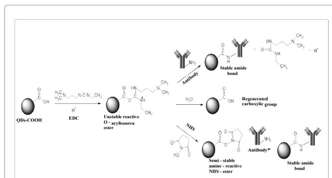
Figure 1: The coupling of Quantum Dots 710 nm to anti-bovine neutrophil elastase antibody by EDC and EDC/NHS method.
